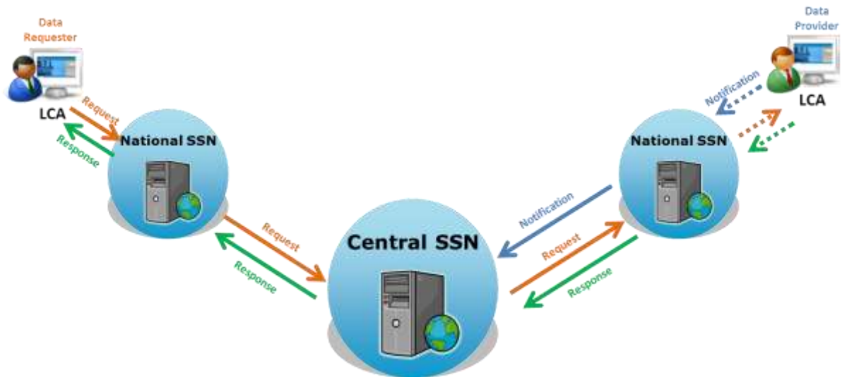
Figure 2 - Sequence diagram of notification, request and response mechanisms
